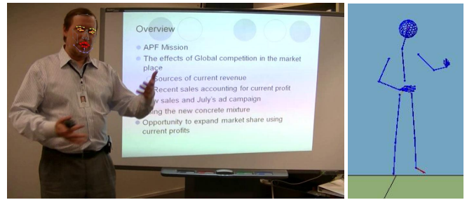
Fig. 1. Multimodal data example (informative speech) : the left panel shows a video of a subject with the tracking of facial features activated; the right panel shows the corresponding motion-trace
